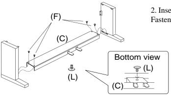
2. Insert the adjuster (L) on Pedal Board (C). Fasten (A) and (C) with four screws (F).
